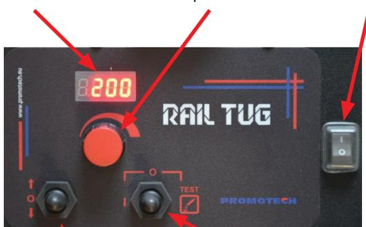
Travel direction switch (Forward/ 0 /Backward)      Arc ignition switch (I / 0 / TEST)
