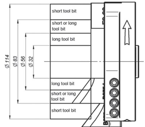
Together with 0° facing tool bit either standard or long beveling tool bits are in use depending on pipe diameter
