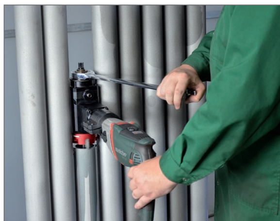
Minimum distance between tubes is 75 mm (2.95")
