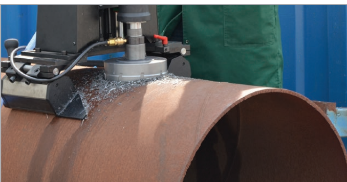
PRO-200A ATEX can be fixed to pipes of min. 950 mm (37.4") diameters
