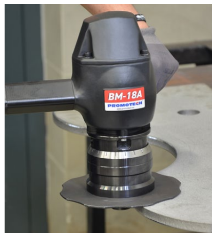
Creating a perfect radius on both straight and curved edges
