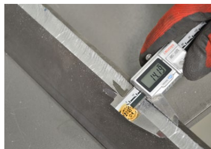
Maximum bevel width up to 14 mm
