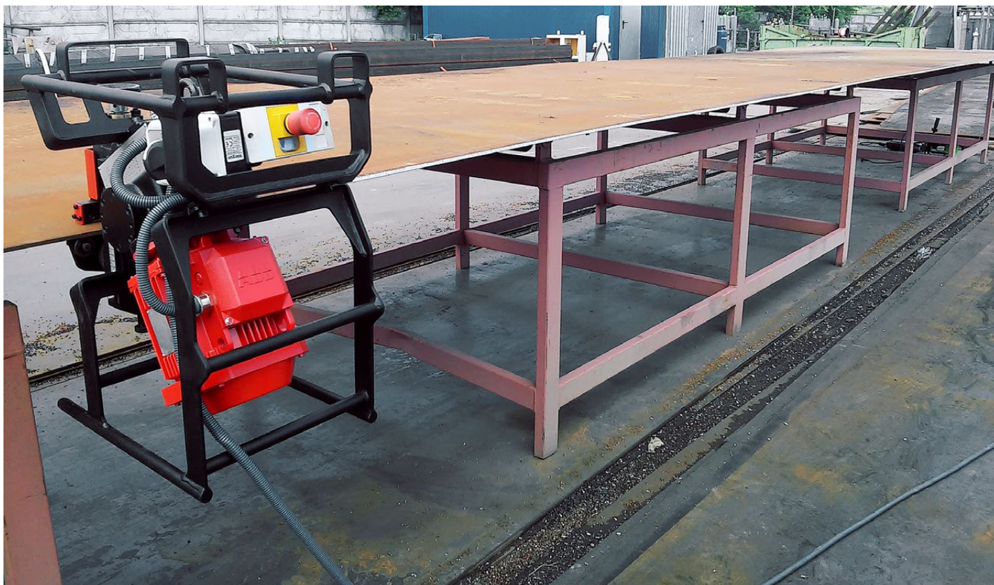
ABM-14 runs along a plate automatically
