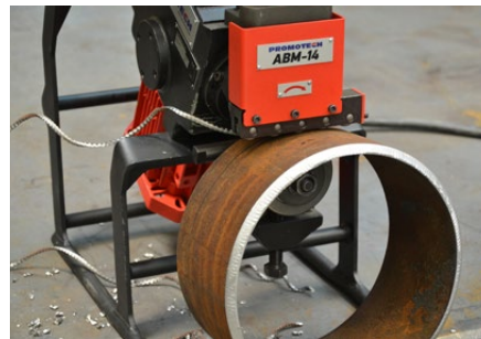
Oval workpiece and pipe beveling
