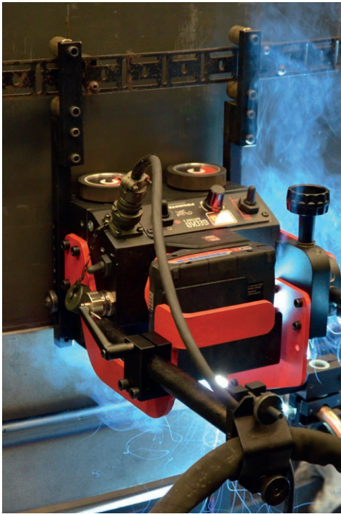
36 mm wide flexible track, length 185cm (6ft) 1pc Minimum curvature radius of 1.0 m (3.3 ft) PRW-0466-50-01-01-0
