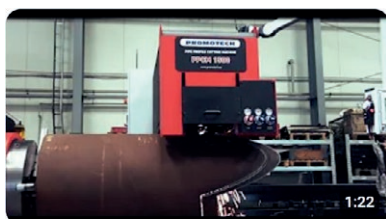
PPCM 1500 - Profile Cutting of 36 Inch Pipe
