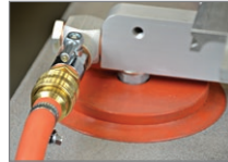
Cut-off valve (for entry vacuum unit) ZWR-0541-10-01-30-0
