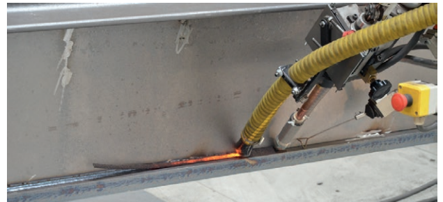
Promotech automatic electro-mechanical joint tracking ensure proper and repeatable welding by means of easy slug removal process.
