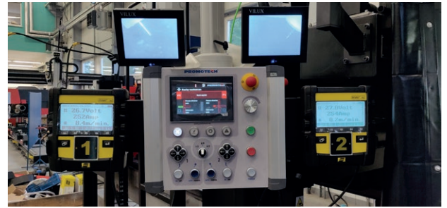
Promotech automatic electro-mechanical joint tracking ensure proper and repeatable welding by means of easy slug removal process.
