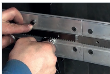
Gear rack adjustment tool. The tool removes the gap between gear racks Product code: PKT-0341-13-00-00-0
