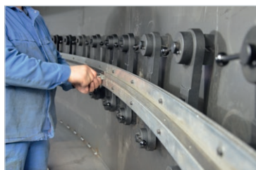
Gear rack adjustment tool. The tool removes the gap between gear racks Product code: PKT-0341-13-00-00-0
