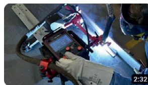
Rail Bull 2 - All position modular mechanized carriage
