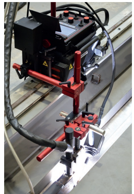
Seam tracking works with and without oscillation
