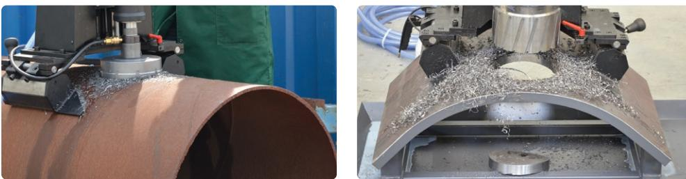
PRO-200A ATEX can be fixed to pipes of min. 950mm (37.4") diameters
