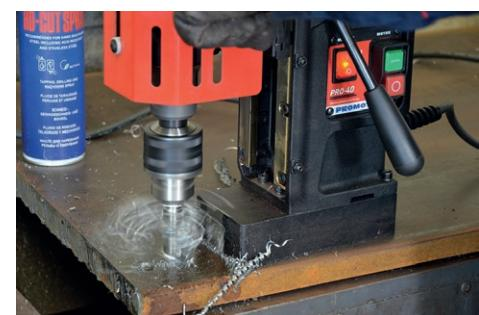
Drilling capacity up to 16 mm (0.63")
