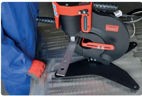
Neither balancer nor hoist arm is required to keep puncher in place. An operator can use start and stop bottoms on the machine or foot pedals.
