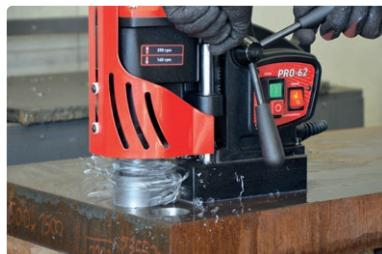
Milling capacity up to 65 mm (2-9/16")
