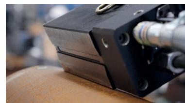
V-shaped prismatic mag base for pipe drilling.
