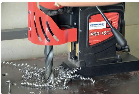
Drilling capacity up to 47 mm (1-7/8")
