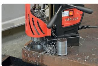
Milling capacity up to 70 mm (2-3/4")
