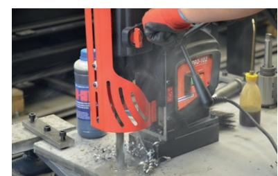
Drilling capacity up to 31.75 mm (1-1/4")
