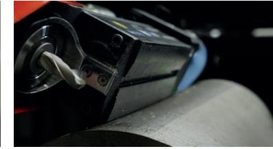
V-shaped prismatic mag base for pipe drilling
