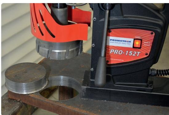
Milling capacity up to 150 mm (5-7/8")
