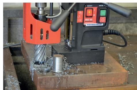
Milling capacity up to 50 mm (2")
