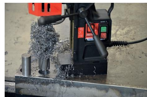
Milling capacity up to 45 mm (2")
