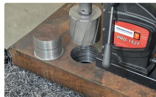
Max depth of cut up to 100 mm (4")
