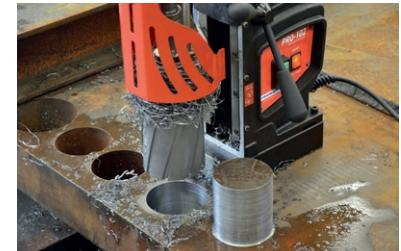
Milling capacity up to 100mm (4")
