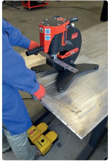
Foot pedal machine control in hands free operation on bench top configuration.
