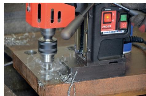
Drilling capacity up to 16 mm (0.63")
