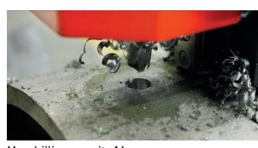
Max drilling capacity 16 mm
