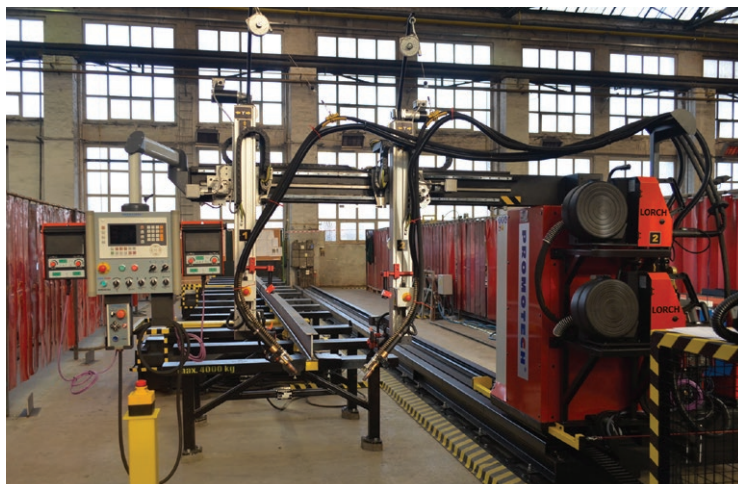
■ GWS type WA MIG / MAG Integrated LINCOLN ELECTRIC PW500 HYPERFILL
