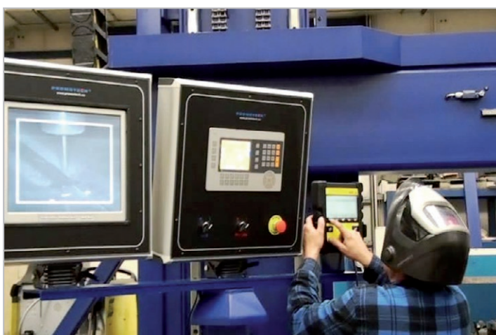
Sample view of CB operating panel and integrated MIG-MAG welding equipment from (ESAB and LORCH)
