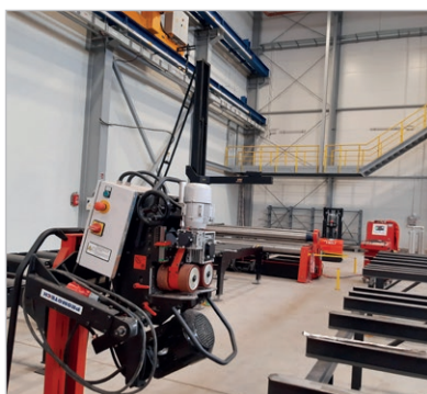
ABM-50 for high-quality single and double-sided bevels
