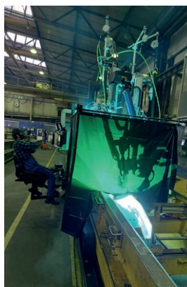
Special design machine for the trailer beam welding.
