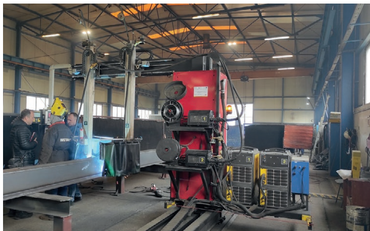
■ GWS type WA MIG / MAG Integrated ESAB ARISTO U5000iw
