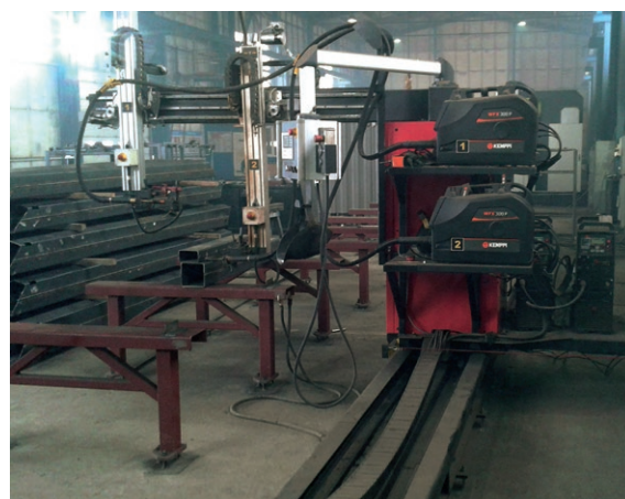
■ GWS type WA MIG / MAG Integrated KEMPPI FASTMIG X 450
