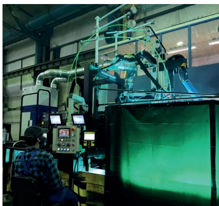
Special design machine for the trailer beam welding.
