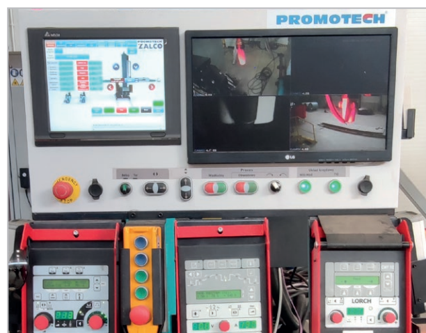
Sample view of CB operating panel and integrated MIG-MAG welding equipment from (ESAB and LORCH)
