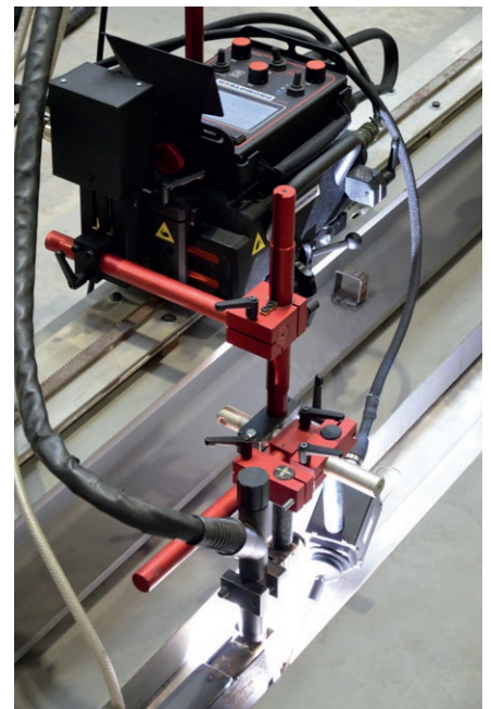
Seam tracking works with and without oscillation
