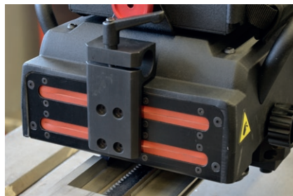
Silicone covers protect against dirt and spatter
