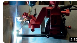
Promotech - Gecko Fillet Welding Carriage
