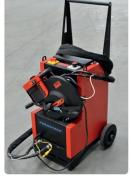
Portable hydraulic power pack with shelf for puncher transport.
