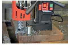
Milling capacity up to 50 mm (2") Depth of cut up to 75 mm (3") - option
