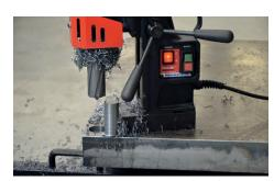
Milling capacity up to 45 mm (1.77") Depth of cut up to 75 mm (3")
