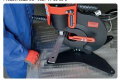
Neither balancer nor hoist arm is required to keep puncher in place. An operator can use start and stop bottoms on the machine or foot pedals.
