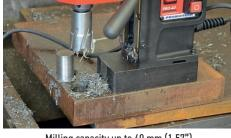
Milling capacity up to 40 mm (1.57") Depth of cut up to 50 mm (2")
