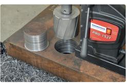
Max depth of cut up to 100 mm (4")
