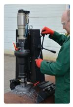
Drilling up to 45 mm (1-3/4")
