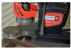
Milling capacity up to 150 mm (5-7/8")
