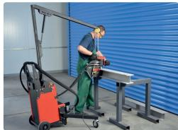
Hoist arm and 2 supports with wheels allow for easy manipulation of punch and power pack as single unit.
