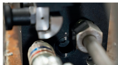
Clamping level indicator for safety and security
