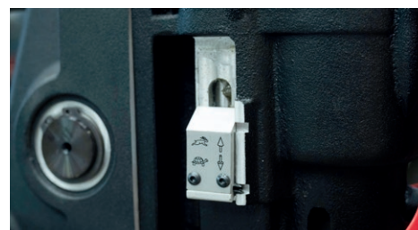
2-gearbox to match the speed to the tool
