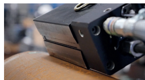
V-shaped prismatic mag base for pipe drilling
