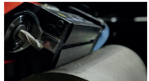
V-shaped prismatic mag base for pipe drilling
