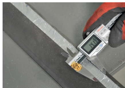
Maximum bevel width up to 14 mm
