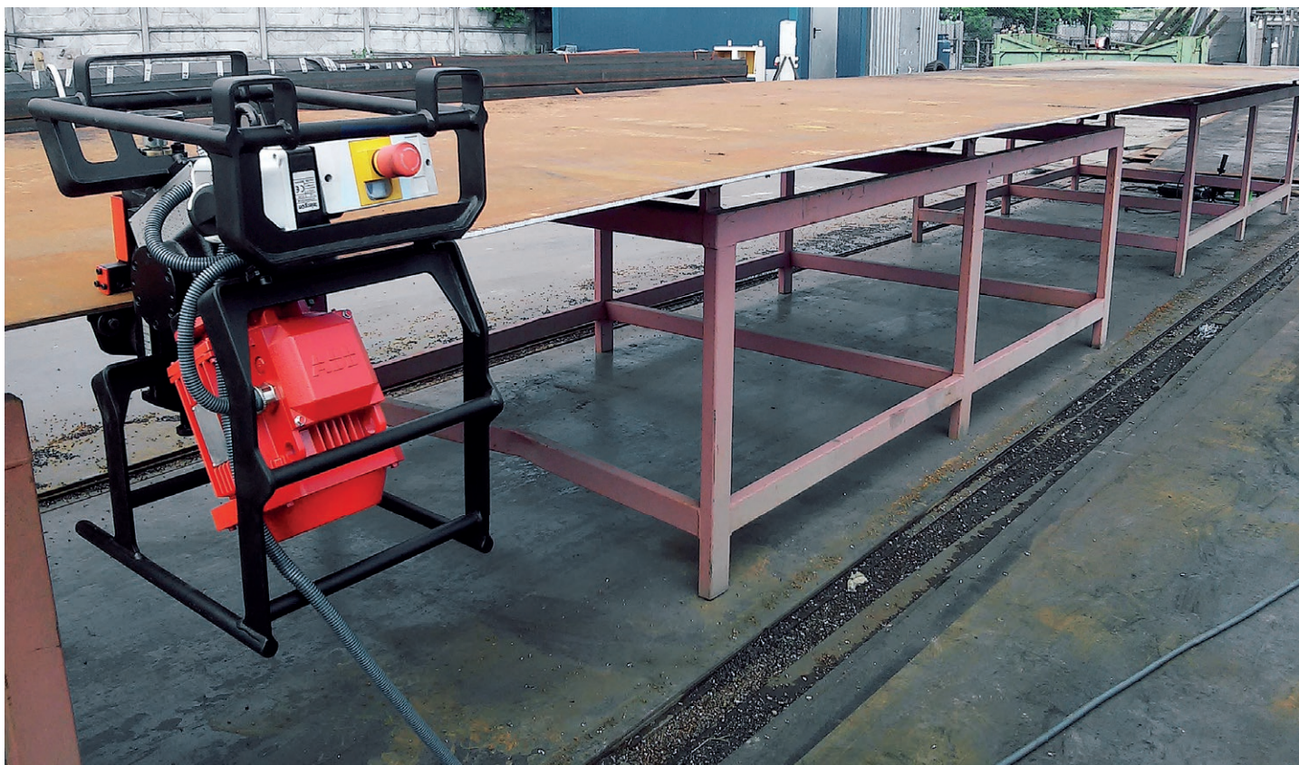
ABM-14 runs along a plate automatically
