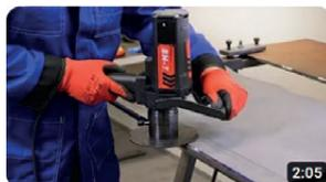
Bm 7 - Compact plate and pipe beveller
