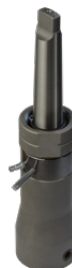
Arbor MT3 x 32 mm Weldon for drilling diameter over 60 mm (2.3") up to 100 mm (4") depth Product code: UCW-0563-22-00-00-0
