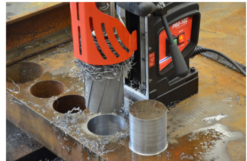
Milling capacity up to 100mm (4") Max depth up to 100 mm (4") Max stroke up to 225 mm (9")
