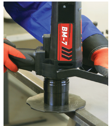
Straight edge beveling with radius
