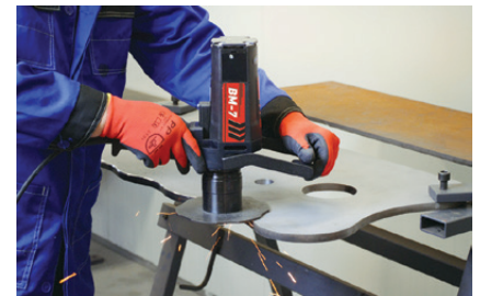
Arched edge beveling with radius
