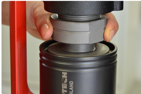
Tapping chuck equipped with securing nut protects tapping tool against pull out
