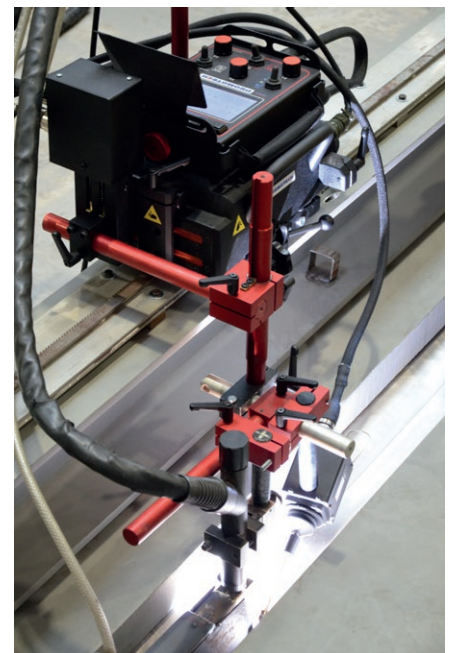
Seam tracking works with and without oscillation
