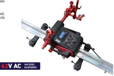
Rail Bull moves along either rigid or semi-flexible track on both ferromagnetic and nonferromagnetic materials thanks to rack and pinion drive and tracks fixed to flat or curved surfaces by means of various magnetic or vacuum units.
