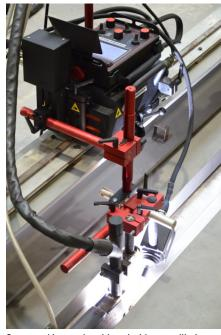
Seam tracking works with and without oscillation
