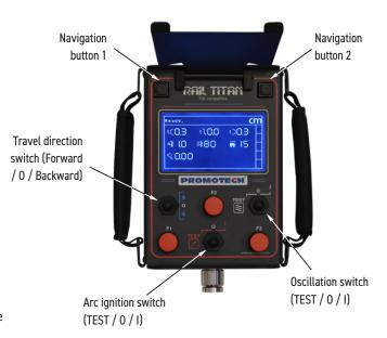
F1, F2, F3 - Rotary parameter/function setting knobs
