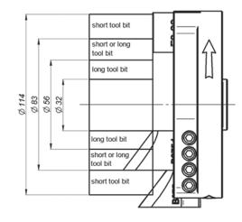
Together with  $0^{\circ}$  facing tool bit either standard or long beveling tool bits are in use depending on pipe diameter
