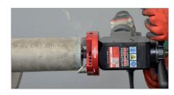
Stainless steel machining is available by means of special tool bits
