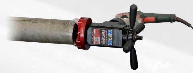
PRO-5 PB is a handy, portable pipe beveling machine suitable for milling edges of pipes made of carbon and stainless steels, aluminum alloys and copper-nickels.
