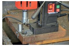
Milling capacity up to 40 mm (1.57") Depth of cut up to 50 mm (2")
