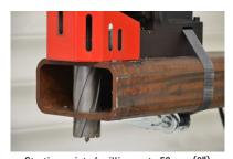
Starting point of milling up to 50 mm (2") below a level of a drill base
