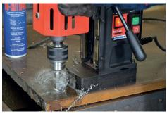
Drilling capacity up to 16 mm (0.63")
