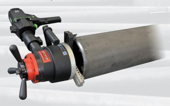
PRO-10 PB is a heavy duty pipe Beveller designed for portable use in pipe machining operations. Self-centering expandable mandrels provide quick and proper alignment to a pipe or a tube prior to machining operations.
