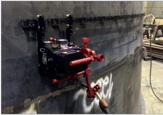
Flexible track length 185cm (6ft) 1pc Minimum curvature radius of 1.0 m (3.3 ft) PRW-0466-50-01-01-0
