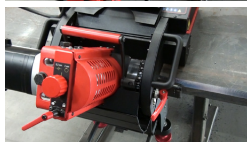
Innovative and ergonomic bevel angle adjustment system with release lever requires no additional tools
