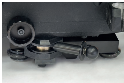
Single lever with lock to position Rail Titan to track
