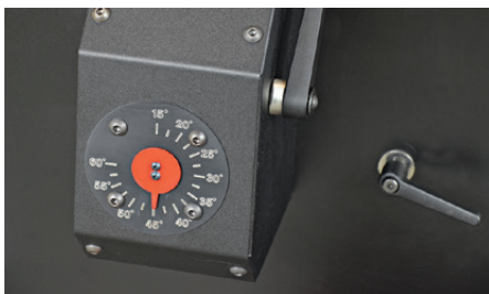
Precise bevel angle adjustment
