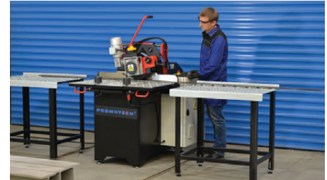
Auxiliary tables to accommodate long workpieces
