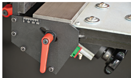
Simple setting of bevel width
