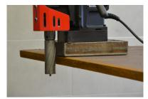
Starting point of drilling up to 50 mm below level of a drill base with 100 mm long cutter
