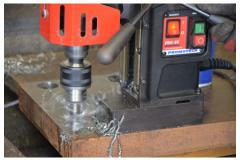
Drilling capacity up to 16 mm (0.63")
