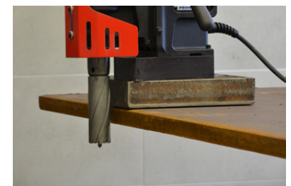
Starting point of drilling up to 50 mm below level of a drill base with 100 mm long cutter
