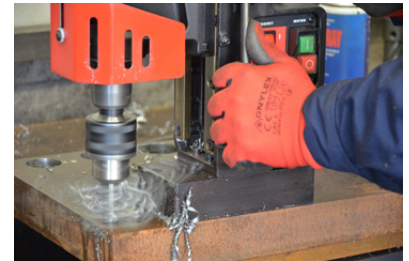
Drilling capacity up to 16 mm (0.63") - with cylindrical shank twist drill in use Drilling capacity up to 23 mm (0.91") - with MT2 shank twist drill in use
