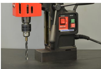
Adapter 3/4" x 1/2" 20 UNF, Drilling chuck 1/2" 20 UNF Twist drills up \Phi 11.8 mm (DIN 338)
