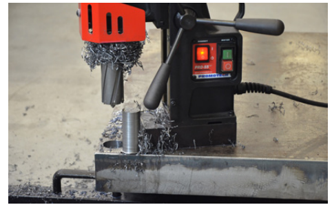
Milling capacity up to 45 mm (1.77") Depth of cut up to 75 mm (3")
