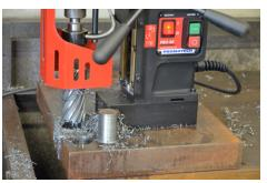
Milling capacity up to 50 mm (2") Depth of cut up to 75 mm (3") - option
