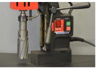
TCT cutters up to  $\Phi$  50 mm with AMT2-C19/2-3 arbor D.O.C. up to 75 mm
