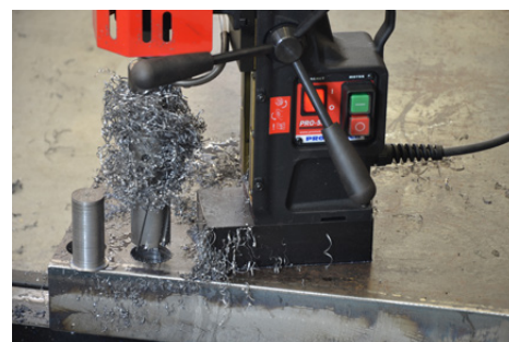
Milling capacity up to 45 mm (1.77") Depth of cut up to 75 mm (3") - option
