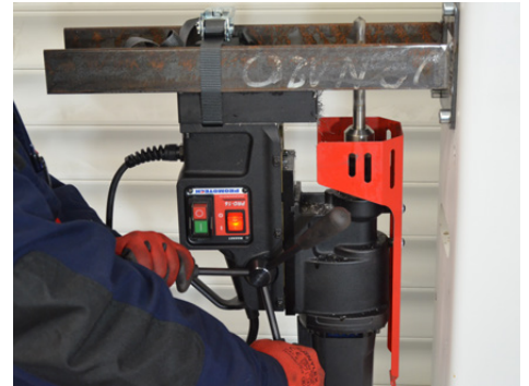
Out of position drilling
