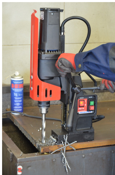
Adapter 3/4" x 1/2" 20 UNF, Drilling chuck 1/2" 20 UNF Twist drills up \Phi 11.8 mm (DIN 338)
