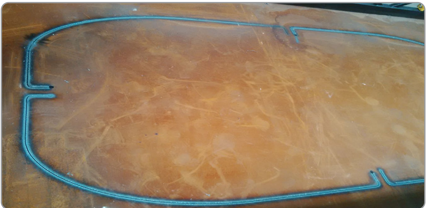
The test of 3D MCM Oxy-cutting prior to final cut at Customer by Promotech Team, plate thickness approx. #80mm.
