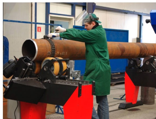
Chain ensures positive axial rotation
