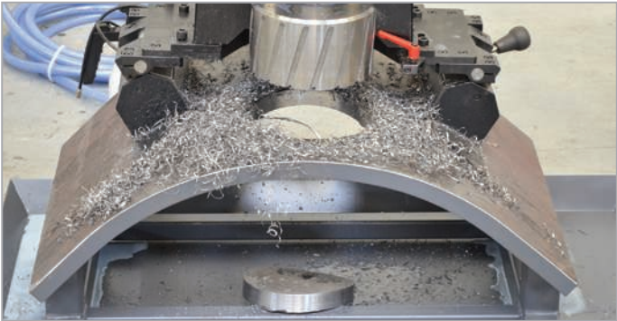
Base with permanent magnets can be adapted to a workpiece curvature
