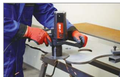
Arched edge beveling with radius
